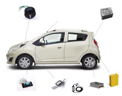
Converting a chevrolet Spark to an electric car begins with the selection of an electric motor, taking into account the weight of the car and the resistance forces acting on it.
