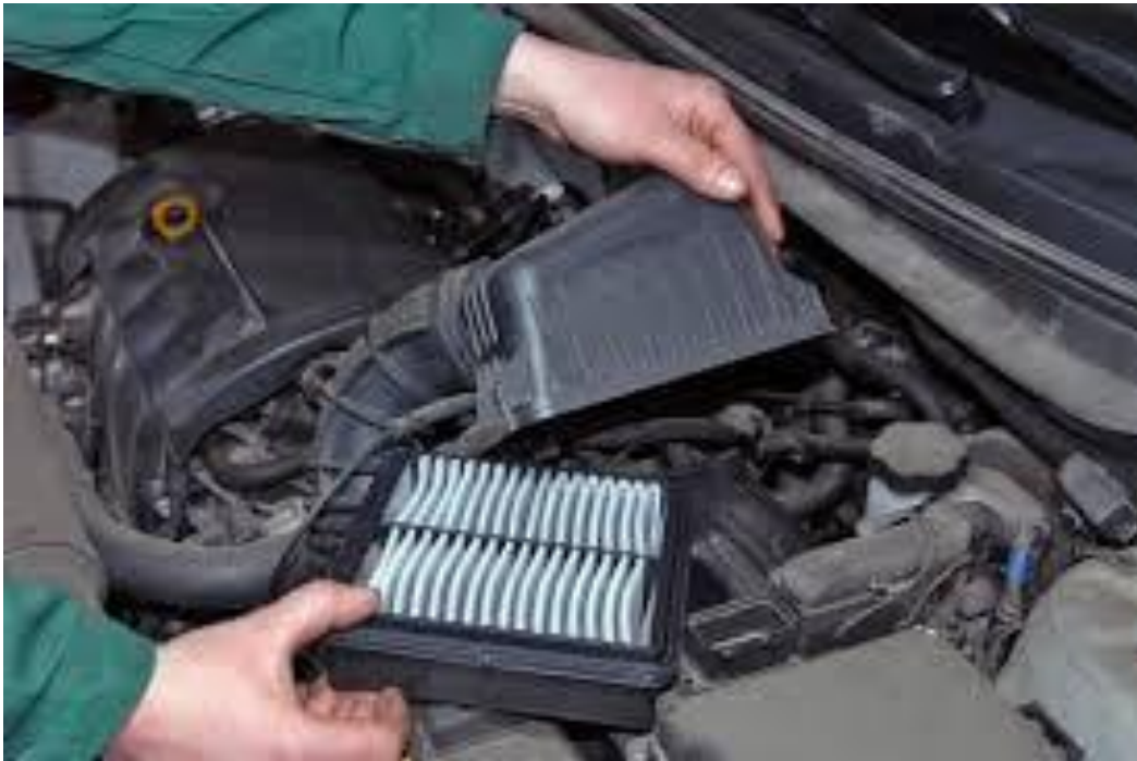
Figure 1. Installation of the air filter in the engine
